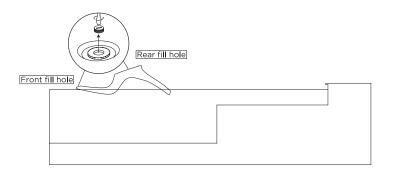
**STEP 2:** Submerge the front fill hole first and allow water to start filling the chaise. You will hear the cavity filling from the base fill hole.
